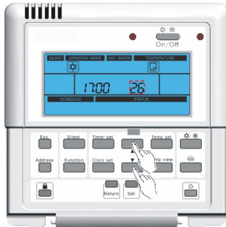
3. Press "Set" to save the adjustment. During operation, press "Return" or "Esc" button to save the set value and return to main interface. The unset items are defaulted to be the last set values.
