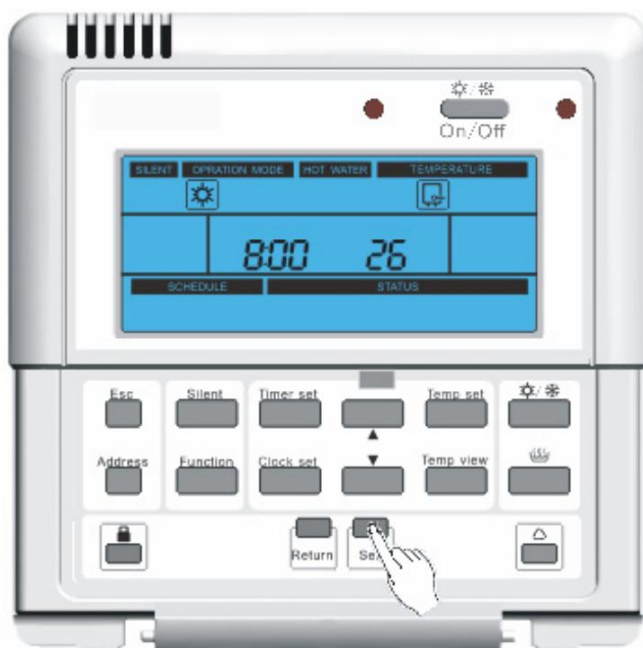
3. and to set timing temperature of the first period. Press “▲” and “▼” button to adjust temperature. Press “Set” to save the adjustment and to set timing temperature of the second period. During operation, press “Return” or “Esc” button to save the set value and return to main interface. The unset items are defaulted to be the last set values.
