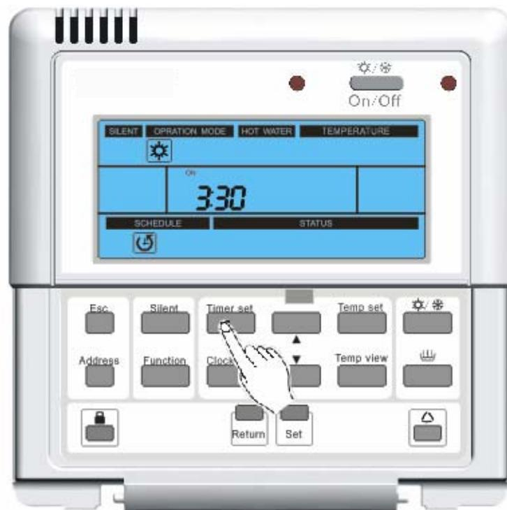
If there is no operation in 20 seconds, the system will exit current setting menu automatically.
