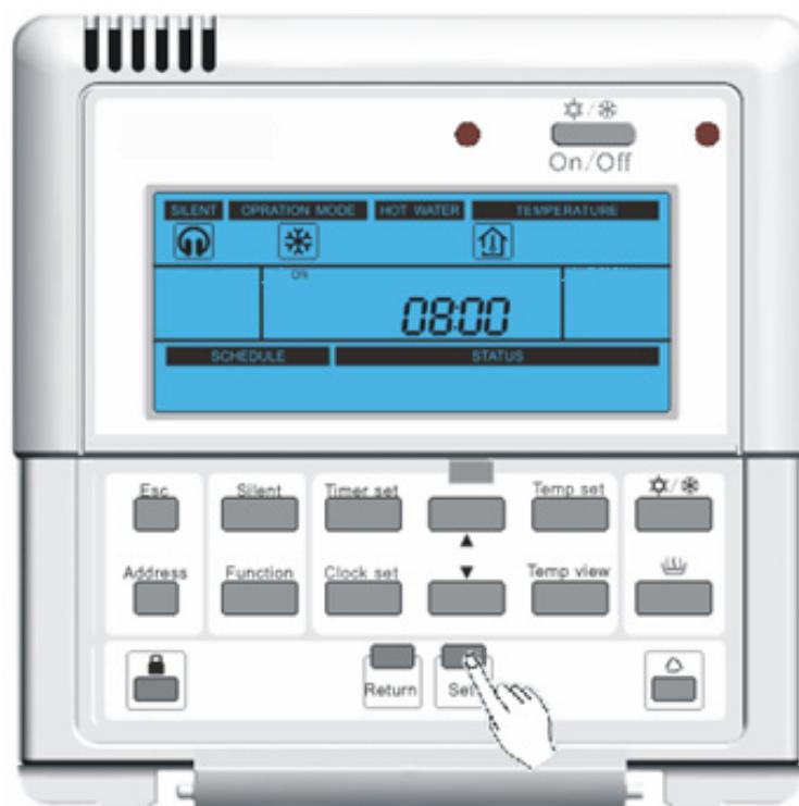
5. During operation, press “**Return**” or “**Esc**” button to save the adjustment and return to main interface. But the timing silent function is not set successfully.
