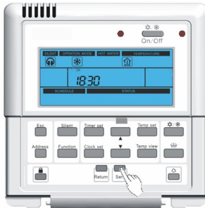
2. Press “▲” and “▼” button to adjust starting minute. Press “Set” button to save the adjustment and to set stopping hour, with “OFF” icon showing.
