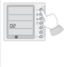
Press and hold the "MODE" key for 10 seconds when the unit is shut off to switch set values so as to decide if the unit operating status or shutoff status shall be memorized after a power fail. If the set temperature area displays 01, it means the unit operating status or shutoff status shall be memorized after a power fail; 02 means the operating status or shutoff status shall not be memorized. Press the "ON/OFF" key to store the set value and exit the setting.
