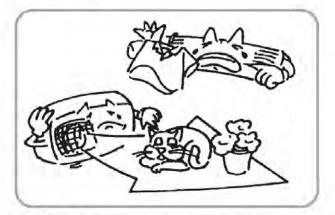
Do not locate a heater or any other heat source close to the unit. The heat may deform plastic parts.
