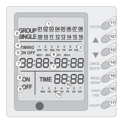
the lower unit. The weekly timing function is able to realized four timing ON/OFF periods for any unit every day, so as to achieve fully automatic operation.
