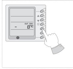
Under normal conditions, the "OUT ENV" column shall only display the indoor temperature. Press the "SLEEP" key for 5 consecutive seconds when the unit is shut off or start up, the LCD shall display "OUT ENV". After the outdoor temperature is displayed for 10 seconds, the system shall return to the display interface of indoor temperature. Note: If not equipped with an outdoor ambient sensor, the unit shall not have this function.
