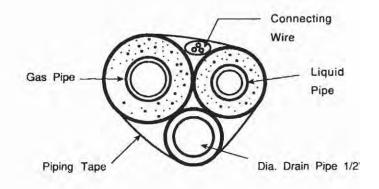
The connection between an indoor unit and an outdoor unit.
