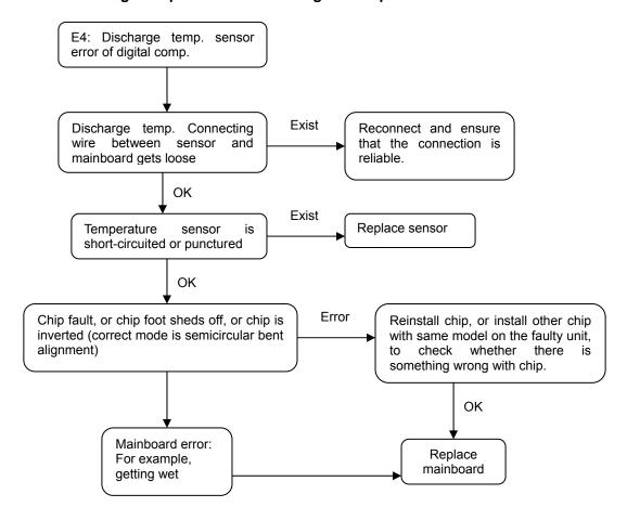
**Case:** Digital Scroll Comp. has two temperature sensors, one is in the compressor, the other one is on the discharge pipe.
