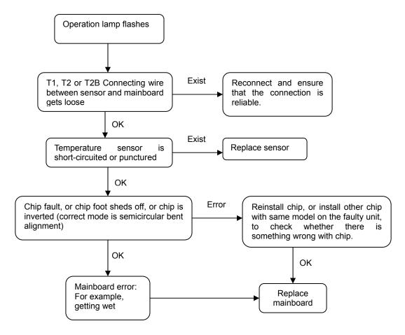
**Caution:** There are three temp. sensors in indoor unit, i.e. T1, T2 and T2B, of which fault in any one will cause operation light flashing and report error.
