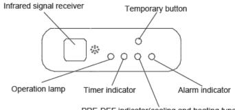
PRE-DEF indicator(cooling and heating type) or fan only indicator(cooling only type)
