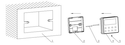
Fig.4 Sketch for Installation of Wired Controller
