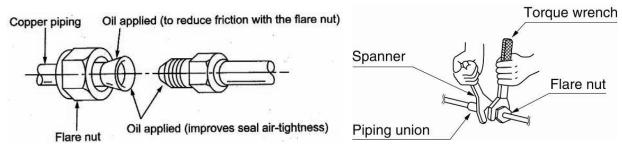
Refer to Table 5 to check if the wrench had been tightened (too tight would mangle the nut and lead leakage).
