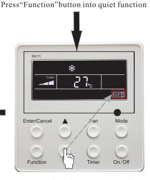
Press"Function"button to turn on the type of quiet function
