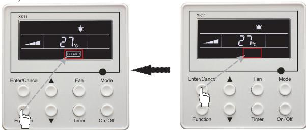
Press"Function"button into E-Heater function
