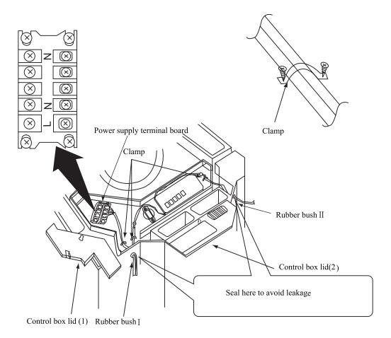
Precautions: Be sure to connect the indoor unit and outdoor unit at right poles.
