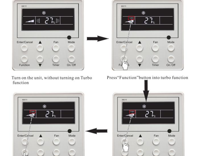
Press"Function"button into turbo function
