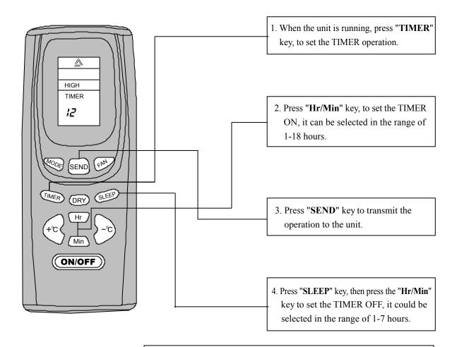
After the SET TIMER ON, the unit turns off at once, when the set time arrived, the unit will run in original mode.
