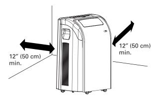
• Place the unit in an area where the temperature will not fall below  $18^{\circ}$ C. The coils will be covered with frost at temperatures below  $18^{\circ}$ C, and this may reduce performance.
