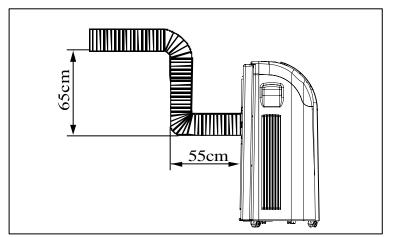
Wrong installation is shown in following figure (If the pipe is bent too much, it would easily cause malfunction.)
