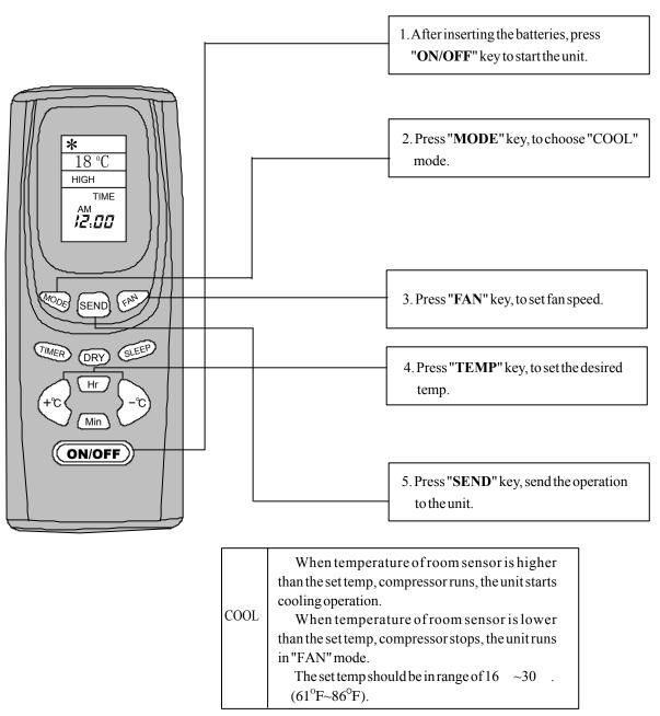
NOTE: When using Fahrenheit remote controller the sign ' ${}^{\circ}$ C', '+ ${}^{\circ}$ C' or '- ${}^{\circ}$ C 'will be corresponding changed to ' ${}^{\circ}$ F','+ ${}^{\circ}$ F' or '- ${}^{\circ}$ F'.
