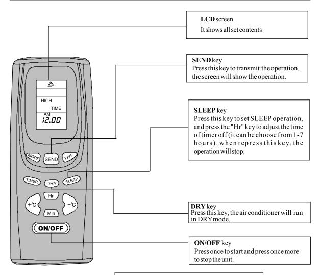
Make sure to aim the signal port of remote controller at the signal receiver indicator of front panel.
