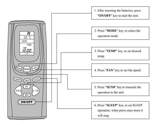
When the unit is running in SLEEP mode, press "Hr" key to set timer on, the interval is 1-7 hours.
