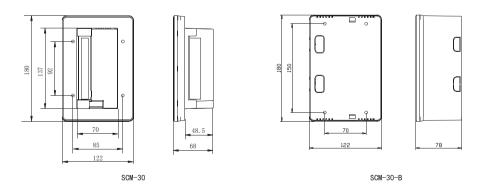
Fig.1.1 Centralized controller size (unit: mm)
