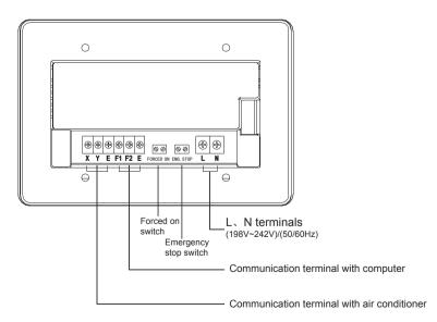
Fig.1.3 Terminal instruction of centralized controller
