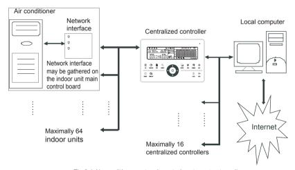
Fig.2.1 Air conditioner network control system structure diagram
