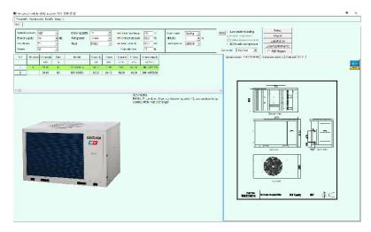
For output you can use a detailed solution performance, CAD drawing (DWG file), EER, COP and also Integrated Part Load Value which means unit performance based on load capacity 25, 50, 75, 100%.
