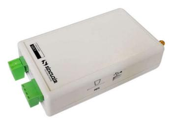
**G2S-T module** G2S-T module is used for remote monitoring of room temperature. When a set temperature is exceeded, the module sends information to user's mobile phone. Hence the module has to be equipped with a mini SIM card in order to secure the operation. G2S-T is a stand-alone device, there is no connection between the module and the air conditioner itself. Therefore you can use our G2S-T module for all kinds of applications including installations with devices of other brands.
