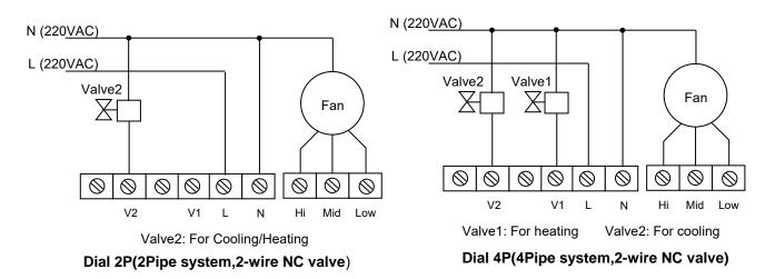
**WIRING DIAGRAMS Attention:** The correct model is compliant with the part number on packing label of controller box; Please check out the correct model and use correct wiring diagram.
