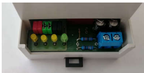
Fig. 7: Jumpers default positions
