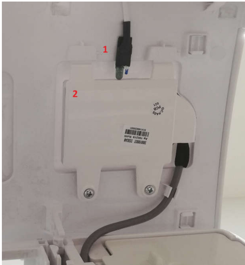
Fig. 3 Location of SC05010 at the indoor unit display – view of the inner side of the front cover
