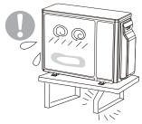
If it is damaged, it may lead to the fall of the unit and cause the injury.
