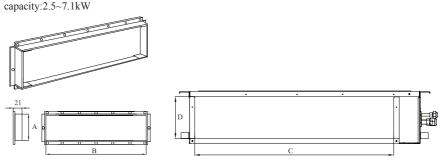
Fig.9 Air Supply Outlet
