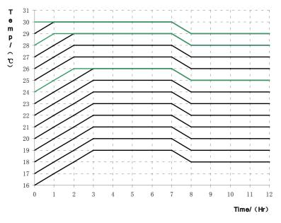
Fig.11 Sleep Curve of Sleep 2 in Cooling Mode
