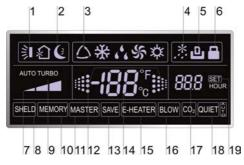
Fig.2 LCD of the Wired Controller
