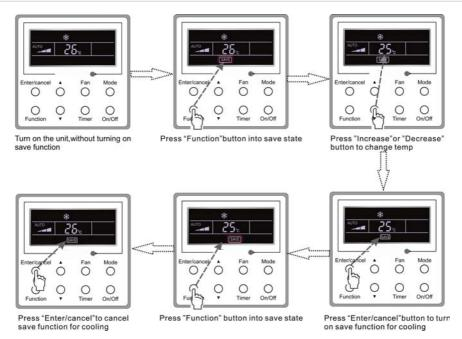
Fig. 15 Saving Setting for Cooling
