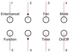
Fig. 3 Buttons on the Wired Controller
