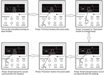
Fig.16 Save Setting for Heating
