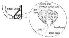
Reserve a certain length of drain hose and power cord for installation when binding them. When binding to a certain degree, separate the indoor power and then separate the drain hose.
