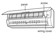
Make the power connection wire go through the cable-cross hole at the back of indoor unit and then pull it out from the front side.
