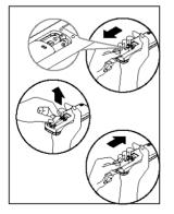
The remote controller is powed by two dry batteries(R03/LR03X2) housed in the rear part and protected by a cover.
