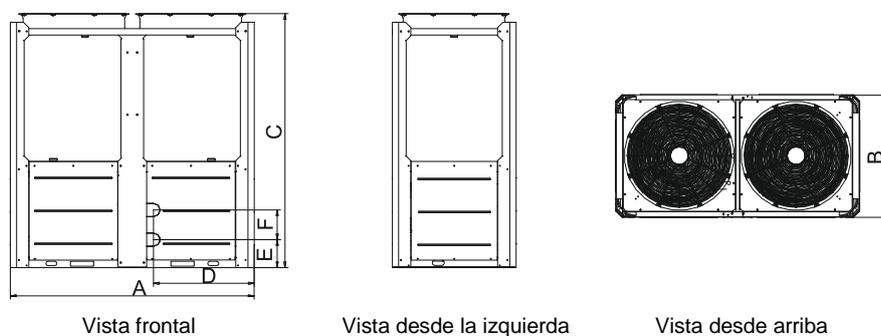
Fig. 6-3 Dimensiones de contorno SCV-900EB
